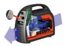
The ICS<sup>TM</sup> (Isolated Cooling System) prevents the dust and the small metal particles from penetrating the machine's interior. The cooling air flows from the back of the machine forward – this minimizes the intake of particle content. Shielded knobs and durable casing makes machine excellent for site jobs.
