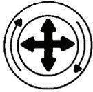
*Rotate the filter while pulling straight out.*
