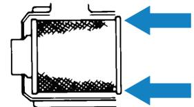
The critical sealing area will stretch slightly, adjust itself and distribute the sealing pressure evenly. To complete a tight seal, apply pressure by hand at the outer rim of the filter, not the flexible center. (Avoid pushing on the center of the urethane end cap.) No cover pressure is required to hold the seal. NEVER use the service cover to push the filter into place! Using the cover to push the filter in could cause damage to the housing, cover fasteners and will void the warranty.
